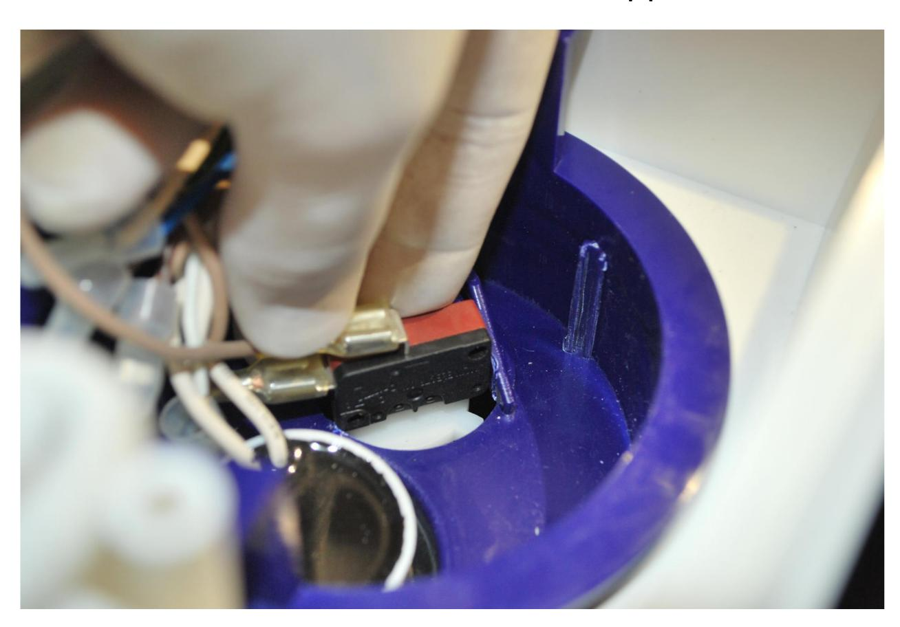
**d.** Disconnect the micro switch fastons and replace it with a new one (T-PF.P120)
