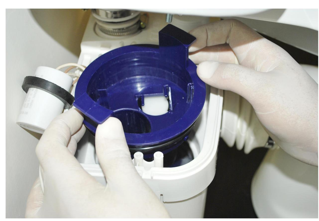
e. Remove the water level switch and clean it using fresh water
